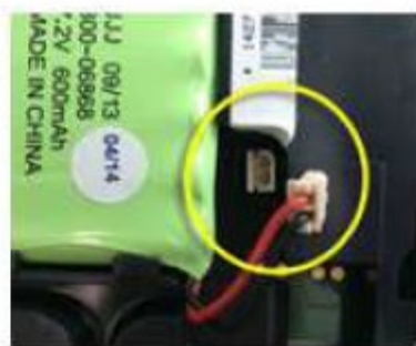
UNPLUG BATTERY PACK FROM UNIT
