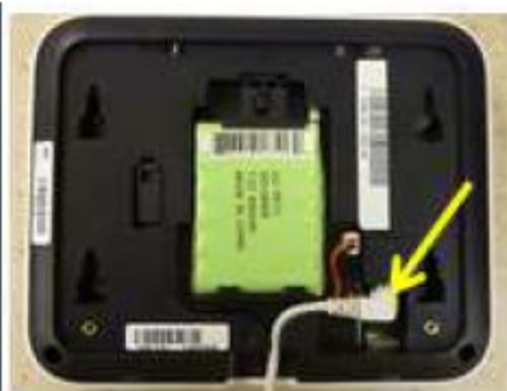
DISCONNECT POWER CABLE. REMOVE MOUNTING PLATE FROM WALL
