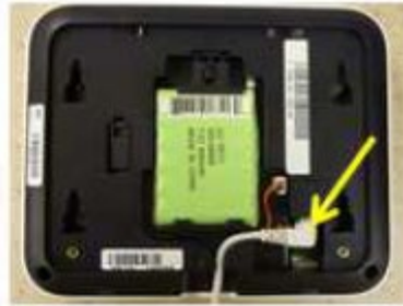
DISCONNECT POWER CABLE
