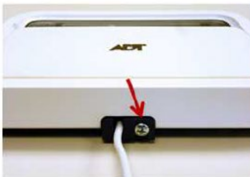
REMOVE RETAINING SCREW ON BOTTOM OF UNIT
