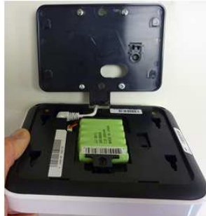
PRESS UPWARDS TO SLIDE THE KEYPAD OFF MOUNTING PLATE
