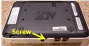
REMOVE RETAINING SCREW
