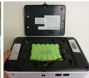
PRESS UPWARDS TO SLIDE BASE UNIT OFF MOUNTING PLATE
