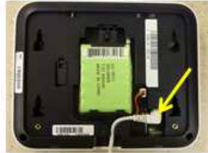
DISCONNECT POWER CABLE. REMOVE MOUNTING PLATE FROM WALL
