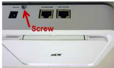
REMOVE RETAINING SCREW
