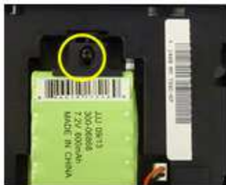
LOOSEN THE SCREW THAT HOLDS BATTERY IN PLACE
