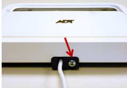
REMOVE RETAINING SCREW ON BOTTOM OF UNIT
