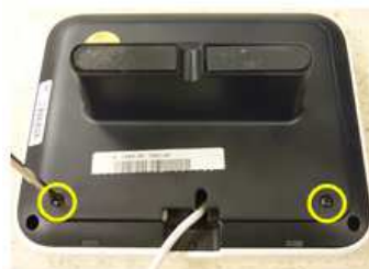
REMOVE SCREWS. LIFT DESK STAND UP AND AWAY FROM KEYPAD
